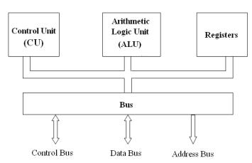
An instruction is fetched from primary storage by the Control Unit; The Control Unit decodes the instruction:
