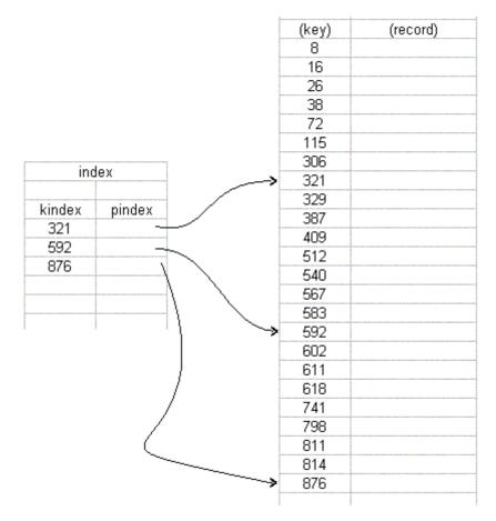
The index file contains a key-index field of only selected data. At a given particular instance, the search is only needed for 321, 592, and 876. The index file also contains a pointer-index that contains the actual address of the keys in the original file. To search the record for key 592, the address is searched in the index file and then the record of the key 592 is directly read from the original file.
