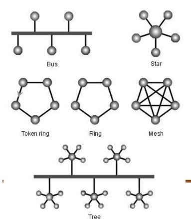
In communication networks, a topology is a usually schematic description of the arrangement of a network, including its nodes and connecting lines. There are two ways of defining network geometry: the physical topology and the logical (or signal) topology.
